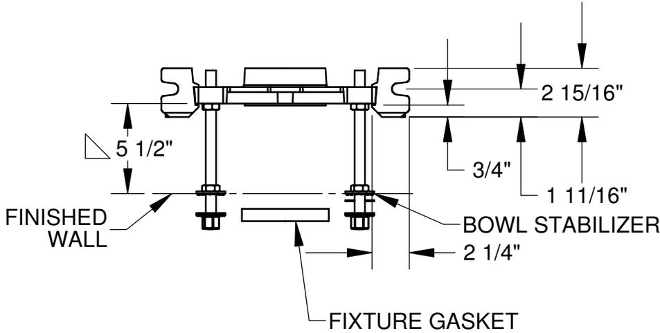
△ FOR DIMENSION SHORTER THAN 5-1/2" (1" MIN) CUT EXTENSION. FOR LONGER EXTENSION (10-1/2" MAX) SPECIFY (-10).
