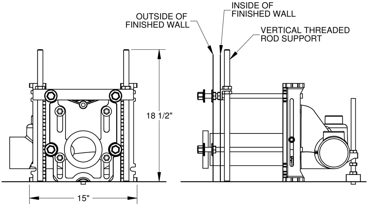
RECOMMEND CONCRETE ANCHORS WITH 750 LBS. PULL-OUT FORCE EACH.
